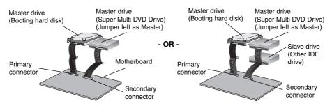
**NOTE :** A hard disk is normally installed as the Primary Master on the EIDE (ATAPI) interface. Other EIDE peripheral devices such as hard drives and Super Multi DVD Drives are then set differently.
